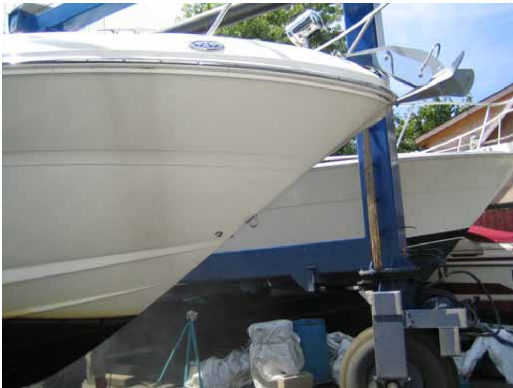
Photo 6. Close-up bow view and plow anchor on stainless roller.
