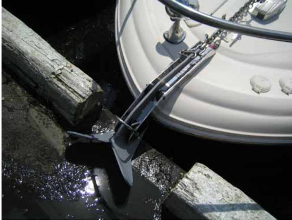
Photo 10. Delta style plow anchor and bracket.
